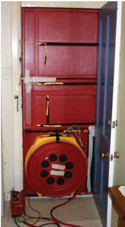
Figure 1: Blower door system used to measure airtightness.
