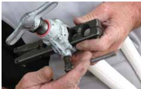
Figure 6.9 Flare the end of the tube (B)
