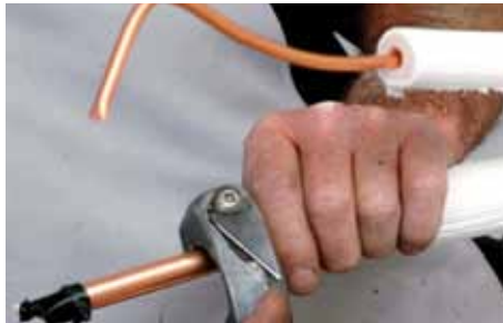
Figure 6.2 Pipe opening facing down when cutting
