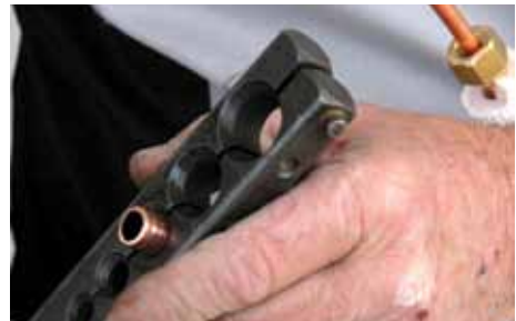
Figure 6.8 Flare the end of the tube (A)
