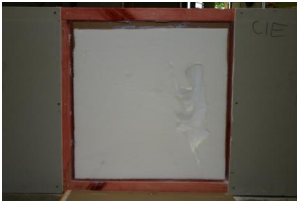
Figure 24: : Shrinkage in low wall C1, specimen C1D.
