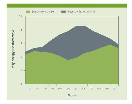
Figure 6.1 The performance of a solar water heater varies throughout the year. The green area is the amount of energy provided by the sun. The grey area is backup electricity provided by the electricity grid.<sup>80</sup>
